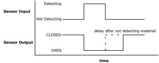
The sensors output is normally CLOSED.
